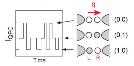
distinguish  $\begin{cases} (1,0) \rightarrow (0,1) \text{ forward tunneling} \\ (0,1) \rightarrow (1,0) \text{ backward tunneling} \end{cases}$
