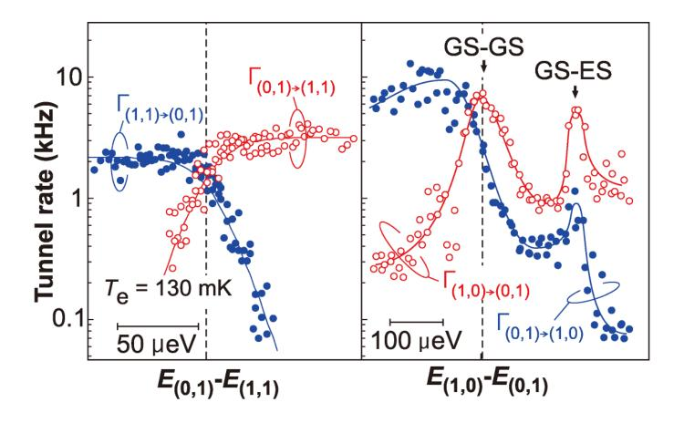
Lead – dot tunneling: broadening ≈ bath temperature
