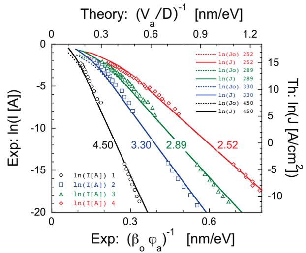
**Figure 2.** Comparison of Fig. 3, Ref. [1] to theory ( $\beta_o = (4516q/cm)$ ,  $D = 10\mu m$ ). Numbers refer to  $\Phi$ .
