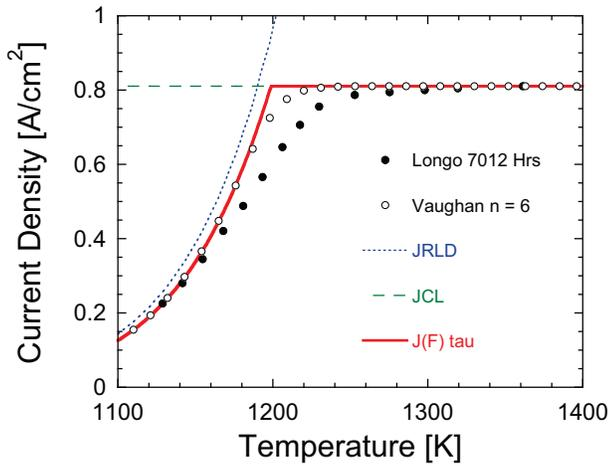
**Figure 1.**  $J(T)$  for Ba dispenser cathode, and an  $\alpha = 6$  curve compared to  $J = J_{RLD}$ ,  $J_{CL}$ , and the transit time model or standard barium dispenser cathodes.
