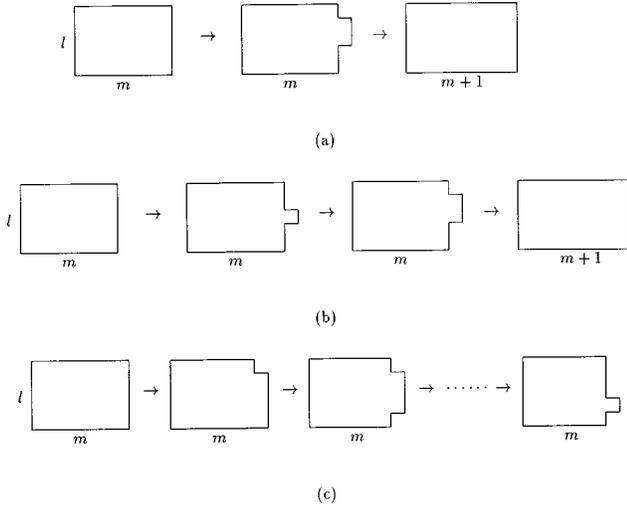
FIG. 2. Growth and shrinking mechanisms: (a) double protuberance growth mechanism, (b) single protuberance growth mechanism, (c) corner erosion.
