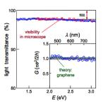
They measure the transparency T of light and from that the conductivity  $T(\omega)=1/[(1+2\pi\sigma(\omega))]^2$  (in the fig. called  $G((\omega))$ ). Between 2 and 3 eV  $\frac{\sigma(\omega)}{\sigma_0}=1.01\pm0.03$
